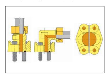
The SAE flange couplings are supplied in standard and high-pressure designs with hole patters in accordance with SAE J 518 or ISO 6162.
