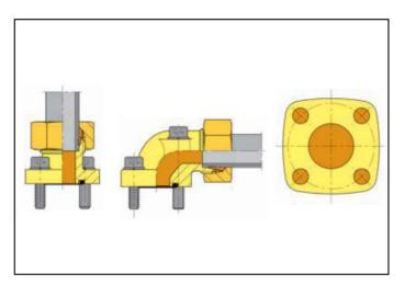
The flange couplings with a square flange connection are characterized by particularly compact outside dimensions. They are supplied in straight and elbow designs. The product range consists of the outside tube diameters from 10 mm to 35 mm. Flange sealing is carried out with an elastic round sealing ring (O-ring), and the mounting connection with cheese head screws. The flange connections are designed for the connection hole patterns of leading pump manufacturers.
