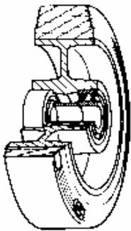
**Tread:** Red non-staining silicone rubber wheels, hardness 80+/-5 Shore A; resistant to temperatures from -30°C and +250°C.
